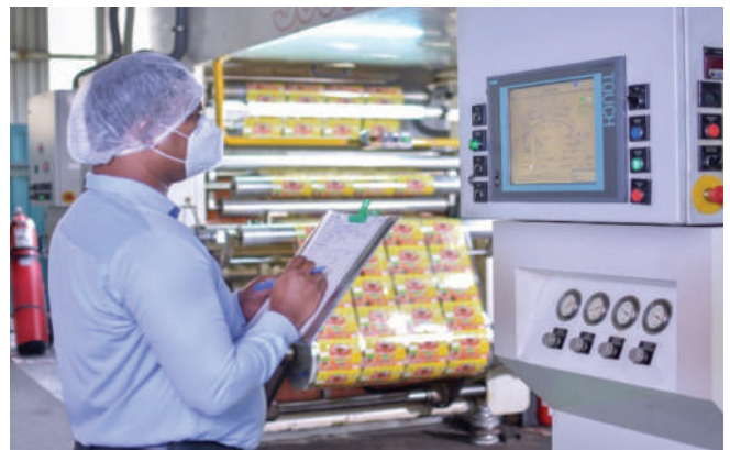
Figure 5.13 – Combi Plaster Film Laminating Machine
