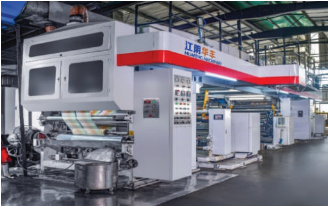
Figure 5.10 – Solvent-Base Laminating Machine Design For Laminating of Plastic Films And Alu-Foil
