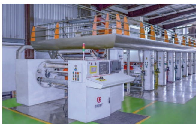
Figure 5.8 – 8 Colour Roto Gravure Printing Machine
